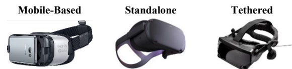
Figure 1. Different Types of VR HMDs (Samsung Gear VR, Oculus Quest, and Valve Index)
