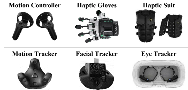
Figure 2. Examples of VR Peripherals (HP Reverb, Manus, bHaptics, HTC Vive Trackers, WorldViz)
