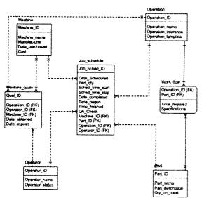
Figure 4: Completed ERD for the Machine Shop
